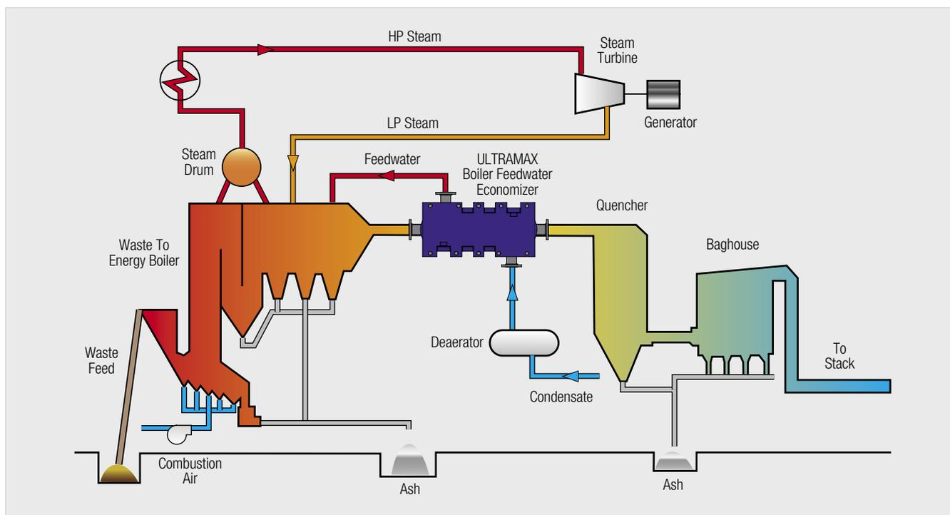
*The ULTRAMAX Welded Plate Heat Exchanger can withstand the corrosive and erosive effects of waste boiler flue gas as an efficiency-boosting feedwater economizer.*
