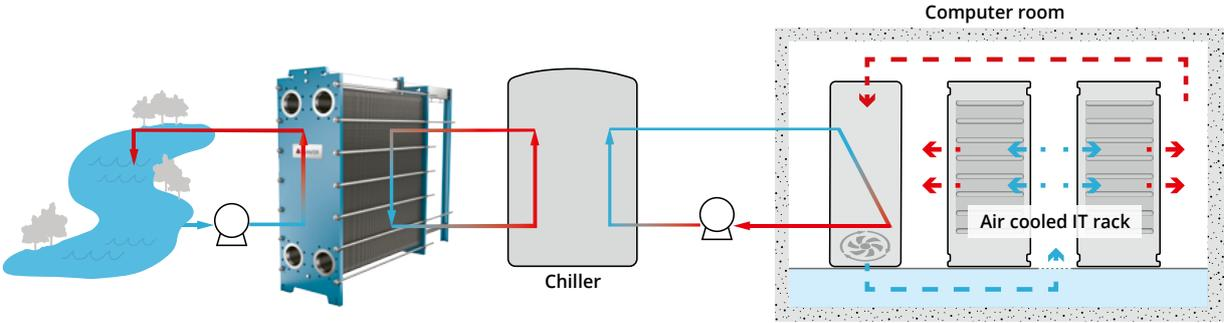
Or by free-cooling from a nearby lake, river or sea. Tranter's plate and frame heat exchangers can be constructed with plates in stainless steel, high alloy or titanium plate material for trouble-free operation, depending on the available cooling source.
