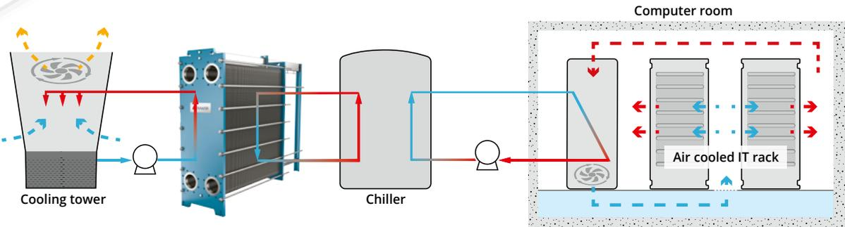
To make the datacenter more sustainable a Tranter plate and frame heat exchanger can be installed as a cooling tower intermediate cooler.
