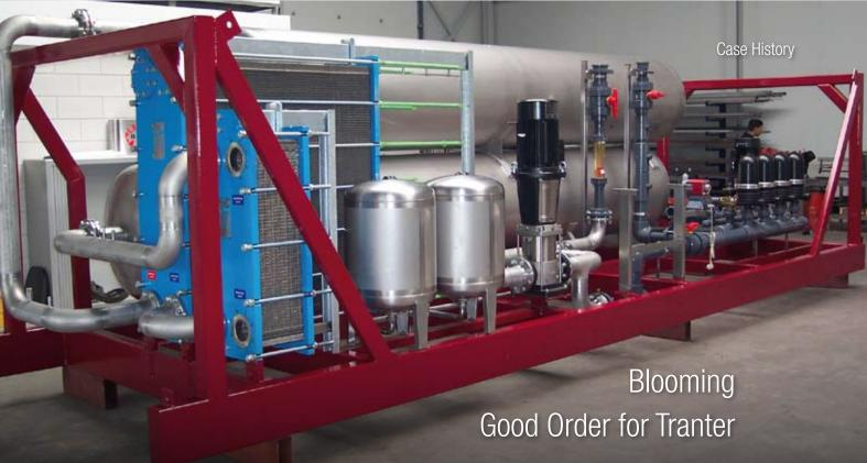
The use of Tranter International AB's plate heat exchangers (PHE) for greenhouse water disinfection equipment is resulting in substantial energy savings for flowers, fruit and vegetable growers around the world.
