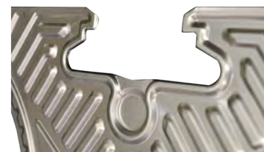
Fig. 5: The Halo™ plate alignment system with a plate-to-plate nesting feature establishes and maintains optimal plate alignment and gasket sealing integrity.
