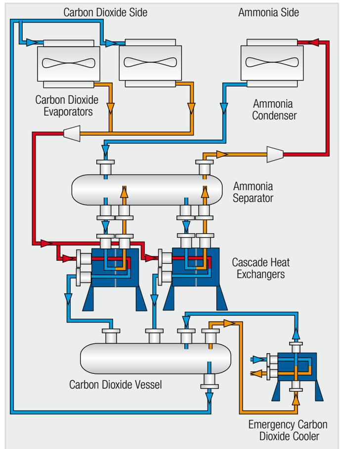
Basics of the NH<sub>3</sub>-CO<sub>2</sub> cascade refrigerating system, with SUPERMAX cascade heat exchangers and CO<sub>2</sub> cooler.
